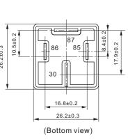
Remark:Terminal vertical deviation tolerance is 0.3mm.
