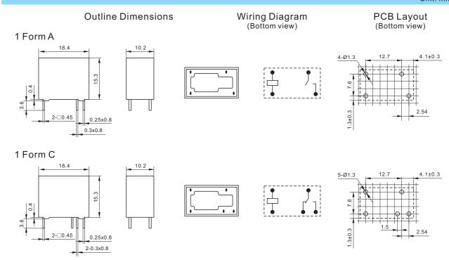
Remark: 1) The pin dimension of the product outline drawing is the size before tinning (it will become larger after tinning), and the mounting hole size is the recommended design size of the PCB board hole. The specific PCB board hole design size can be mapped and adjusted according to the actual producet.
